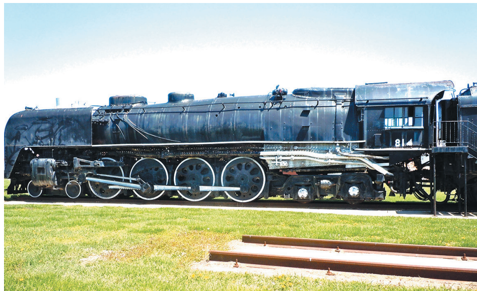
UNION PACIFIC 4-8-4 featuring classic elephant-ear smoke deflectors. By the date of this photo the locomotive was finishing up its last days in freight service.
